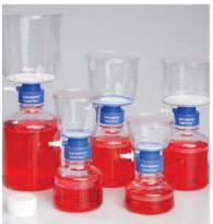
Nalgene™ Rapid-Flow disposable Filter Units with PES (polyethersulfone) membrane provide the last line of defense against cell culture contamination.
