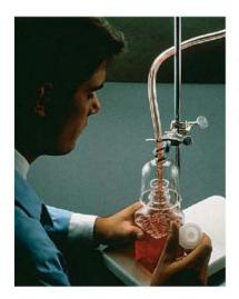
Nalgene™ Polycarbonate Filling Bell is used to transfer sterile media aseptically from large containers to media bottles or culture vessels.
