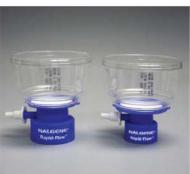
Nalgene™ MF75 disposable Bottle Top Filters with PES (polyethersulfone) membrane provide the last line of defense against cell culture contamination.
