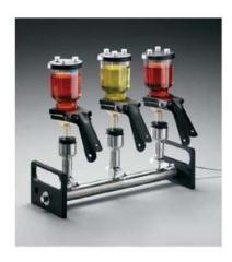
Nalgene™ Reusable Filter Funnels with Clamps are ideal for labs doing high-throughput particle and microbiological QC testing.
