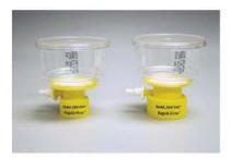
Nalgene<sup>™</sup> Rapid-Flow<sup>™</sup> Sterile Disposable Bottle-Top Filters fit Nalgene filter receiver bottles (#455-series) or standard glass media bottles.
