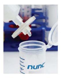
Nalgene™ Syringe Prefilter can clarify small volumes of highly viscous solutions and remove large particulates from suspensions.
