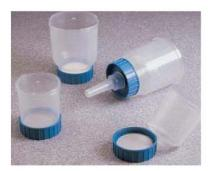
Nalgene™ Sterile Analytical Test Filter Funnels are economical, sterile disposable funnels for microbiological QC testing and analysis of water, food/beverage, raw material and finished product.
