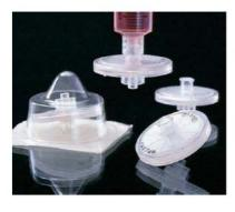
Nalgene™ Syringe Prefilter Plus provides two-stage filtration for sterilization of highly viscous solutions or solutions with high particulate loads. The filter and prefilter membranes are combined in one disposable unit.
