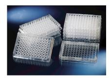
UV transparent 96-well microplates are ideal for DNA and protein quantitation in 260 nm and 280 nm range.
