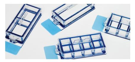
Nunc<sup>™</sup> Lab-Tek<sup>™</sup> II CC2<sup>™</sup> Chamber Slide<sup>™</sup> System is an enhanced version of the Nunc Lab-Tek II Chamber Slide System – enabling cell growth directly on a glass microscope slide. The CC2 surface mimics PDL coating.
