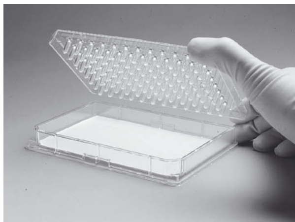
Fig. 1 - By using the disposable TSP 96 Pin Replicator all individual colonies of a plate are replicated on a nylon hybridization filter (e.g. Pall Biotodyne B Nylon Membrane).
